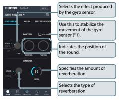
You can automatically position the sound using the gyro sensor built into the WAZA-AIR, and adjust the ambience sound effect.
